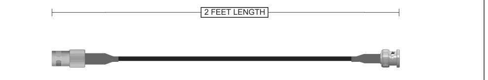
Connector A 112144 BNC Jack Straight Brass Nickel + Heatshrink 50 Ohm RG-58 Continuity/Hi-Pot Connector B 031-320 BNC Plug Straight Brass Nickel + Heatshrink
